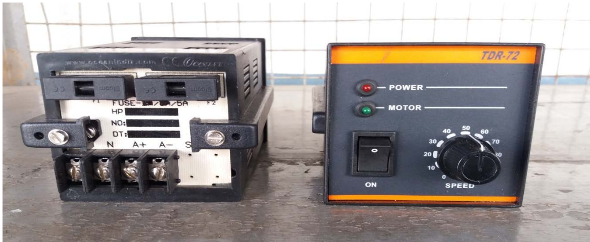
FIG. 3 DC DRIVES FOR PMDC MOTORS
