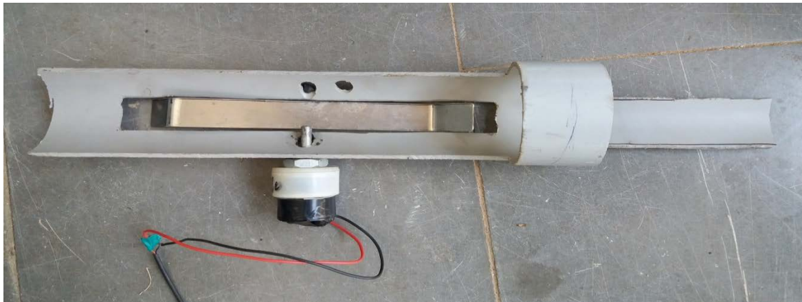
FIG. 5 BALL HOLDER WITH STEPPER MOTOR
